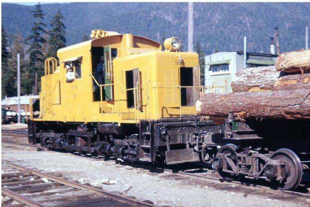
CFP 98 (later renumbered 251) one-of-a-kind diesel shay! 400 hp Cummins. Built 1951 by Tye Machinery, Vancouver using components of steam Shay locomotive.
